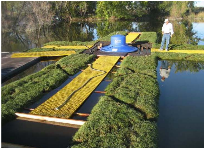
Leviathan Water Circulation System, August 2010 (5000 ft 2 of FTW surface area = 29 acres of effective surface area)
